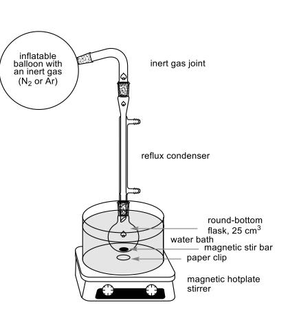
Figure P7. Apparatus for drying of isopropyl alcohol.
