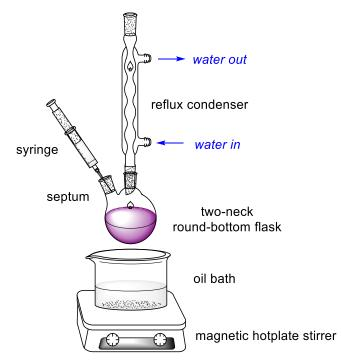
Figure P8. Adding iodoethane by syringe.
