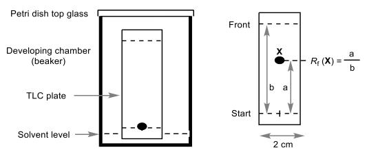
**Figure P6.** Developing a TLC plate (left), evaluation of *R*<sup>f</sup> value (right).
