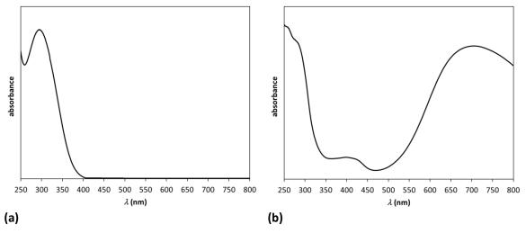
**Figure 3.** Spectra of  $FeCI_3$  and  $Fe_4[Fe(CN)_6]_3$  (in unknown order).
