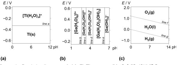
**Figure 1.** Pourbaix diagrams of (a) TI<sup>+</sup>/TI system, (b)  $Ga^{3+}/[Ga(OH)_n]^{(3-n)+}$  system and (c)  $H_2/H_2O/O_2$  system.
